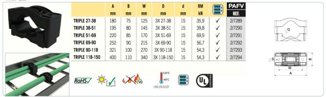
**BASOR Triple cable clamps** are specially designed for short-circuit resistant fastening of of cables in trefoil applications. Triple types are available in 6 models and suitable for cables with a diameter from 27 mm to 150 mm.
